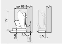
Cabinet front edge to centre of mounting plate drilling 21.5 mm + front thickness FD with mounting plate A20 38.5 mm + front thickness FD with mounting plate A37
